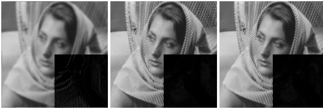
Fig. 1. Examples of image deblurring (Image 'Barbara' 256x256, From left to right: blurred image, Gaussian blur (kernel 25x25, std = 1.6); noise added variance 2; deblurring by GSR , PSNR = 28.26 dB, deblurring by our method, PSNR = 28.76 dB. In lower right corners the differences between deblurred and original image fragments are shown)
