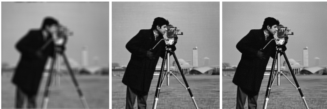
Fig. 2. Examples of image deblurring (Image 'cameraman' 256x256, From left to right: blurred image, uniform blur (kernel 9x9), noise added BSNR = 40 db; deblurring by IDD-BM3D , PSNR = 31.22 dB, deblurring by our method, PSNR = 31.36 dB)
