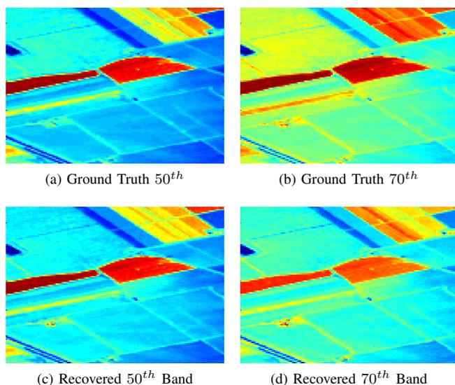
Fig. 3: In this experiment, the high resolution hypercube is estimated from only 6 input spectral observations. The PSNR metric for the recovery of the 3D hyper-cube is **20.36** db. We observe that the reconstructed spectral bands present a faithful representation with the ground truth observations.
