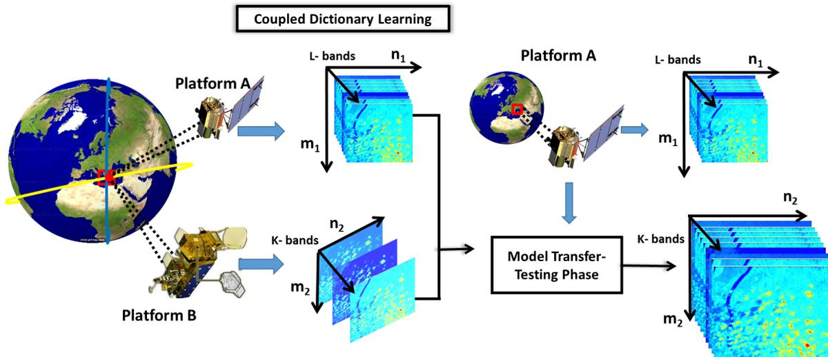
Fig. 1: Proposed Block Diagram: Our algorithm takes as input a 3D data-cube acquired with a limited spatial resolution from Platform A, and utilizes the high-spatial resolution trained model from Platform B, to increase spatial resolution. Respectively, the high-spectral resolution learned model from Platform B is utilized as prior knowledge to enhance the limited spectral information of Platform A.
